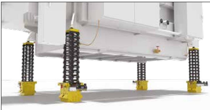
▼ Typical set-up with 4 Self-Locking Cube Jacks and cribbing blocks to lift a transformer (hydraulic power pack and hoses not shown).
